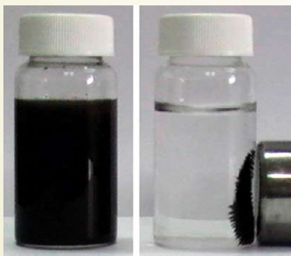
Magnetite-RGO composite dispersed water solution (left) and magnetic separation. [Credit: ACS Nano]
